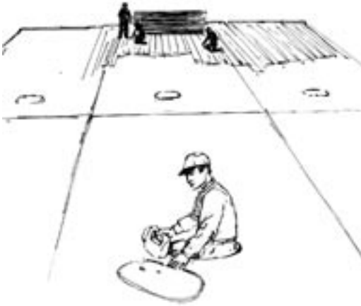
The flotation compartment of a barge is a confined space that may not have enough oxygen to sustain life.
