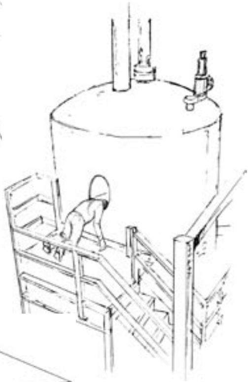
This process vessel at a pulp mill is a confined space. One worker died inside the vessel from lack of oxygen and another died while breathing the air through the opening.
